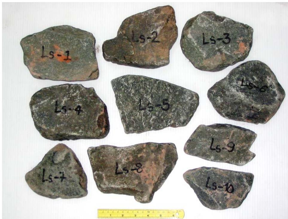
Appendix B-10 Characteristics of ten rock specimens of Lom Sak volcanic complex (lithologic unit Ls) after point load testing
