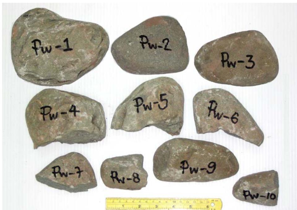
Appendix B-6 Characteristics of ten rock specimens of Phra Wihan sandstone/siltstone (lithologic unit Pw) after point load testing
