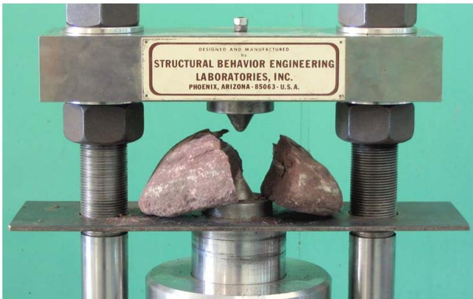
Appendix B-5 Characteristics of ten rock specimens of Phra Wihan sandstone/siltstone (lithologic unit Pw) before point load testing
