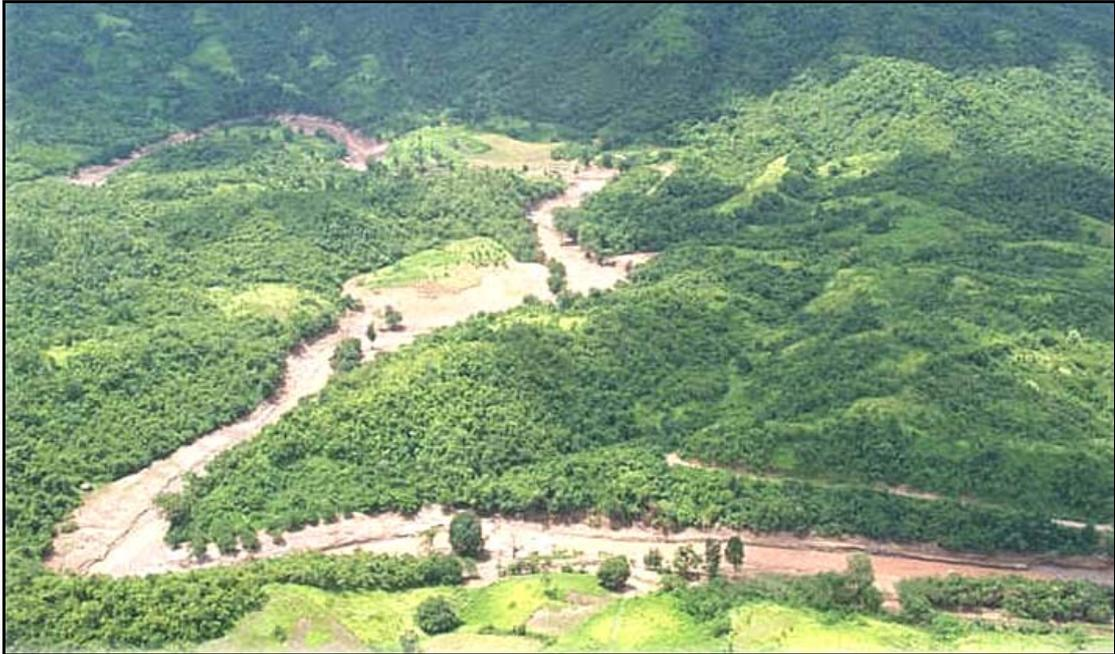
Figure 5-15 Oblique aerial photographs along Nam Ko Yai stream channel. The photograph, at location Z in Figure 5-11, illustrates the flow-flood track along plant debris and soils had been strongly eroded and transported from its banks before reaching the outlet of the Nam Ko Yai sub-catchment.
