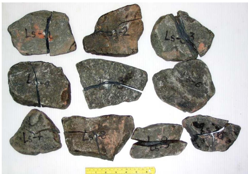
Appendix B-11 Results of point load index strength test of rock specimens of Phra Wihan sandstone (Pw)
