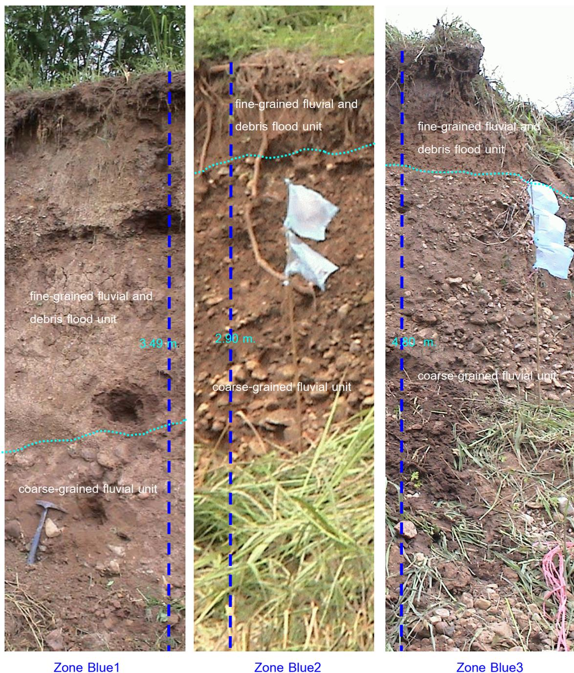
Figure 6-15 Photographs illustrating detailed sedimentary and stratigraphic characteristics in vertical succession of the fine-grained fluvial and debris flood unit that overlay with the sharp contact manner on top of the coarse-grained fluvial unit at the zones Blue1, Blue2 and Blue3.
